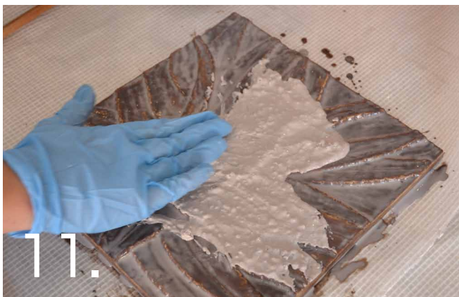
11. Spread the Mould Rubber mix over the panel until the entire object is covered, including the sides.
