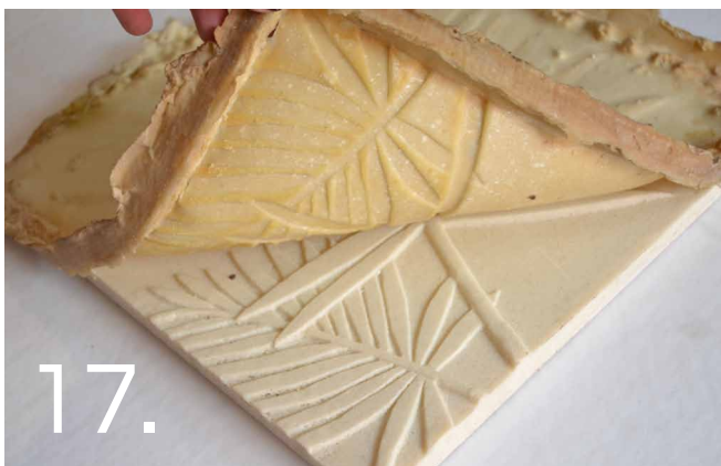
17. Once set, slowly start at the corners and pull the mould away from the panel.
