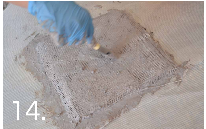
14. You may add additional Mould Rubber to ensure the CemForce is saturated.
