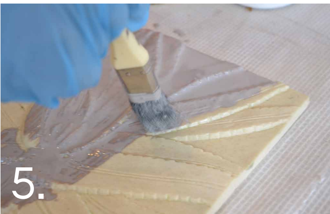
5. Use a brush to spread a thin coat of Mould Rubber over the panel so that it may pick up fine detail. Apply the Mould Rubber at thicknesses of around 3 - 4mm at a time.
