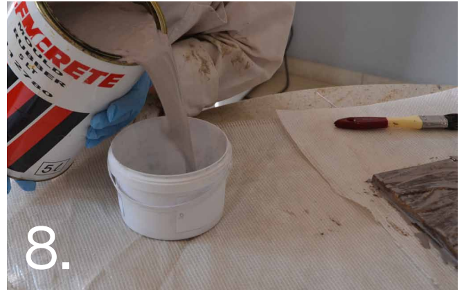
8. Pour some Mould Rubber into a tub. The amount is determined by the size of the panel / object.
