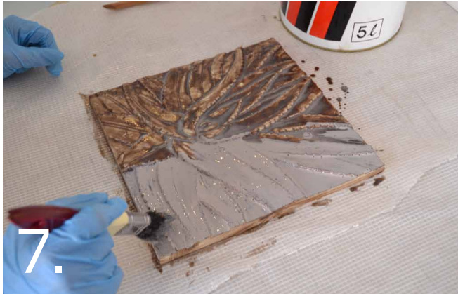
7. Spread another thin (3 - 4mm) coat of Mould Rubber over the first layer and wait for it to dry (it will change colour as it dries.)
