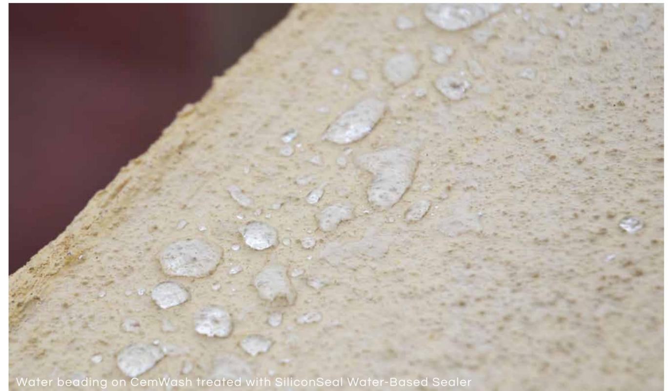
Water beading on CemWash treated with SiliconSeal Water-Based Sealer
