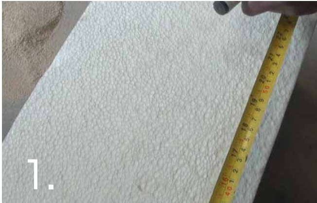
1. Measure and cut the polystyrene to the desired shape and size. Keep in mind that the finished object will turn out a little bigger due to the various preparation and finishing layers.
