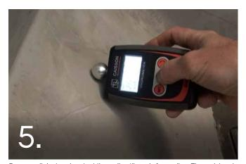
Remove all dust and protect the wall until ready for sealing. The moisture in the wall must be less than 5% before sealing.
