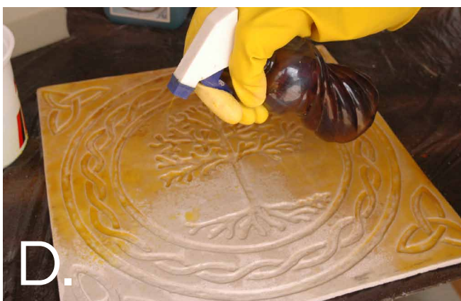
D. Before sealing, the SculptCrete piece can be stained with Cemcrete's CreteStain. Once dry, seal using an appropriate Cemcrete Sealer in accordance with it's datasheet.
