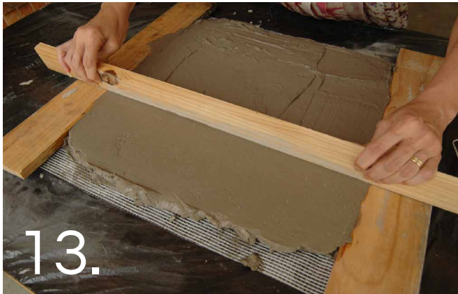
13. Use a piece of wood to level the surface. Press against the wood on the side and draw firmly to scrape the top away.
