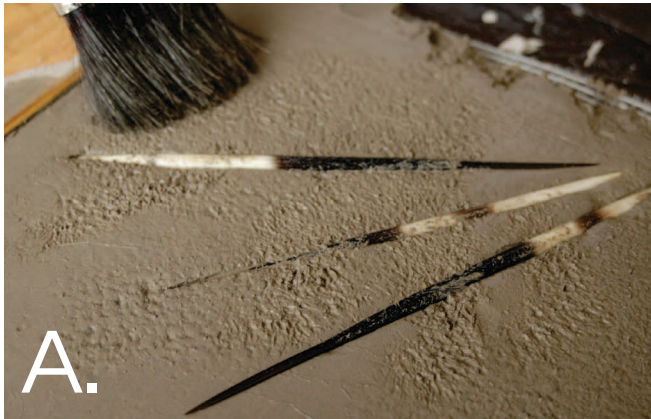
A. Many objects can be embedded into the SculptCrete for various effects and finishes. The SculptCrete can also be textured with a brush, sponge, etc.
