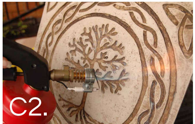
C2. ... and then burnt with a torch for a darker rich finish.
