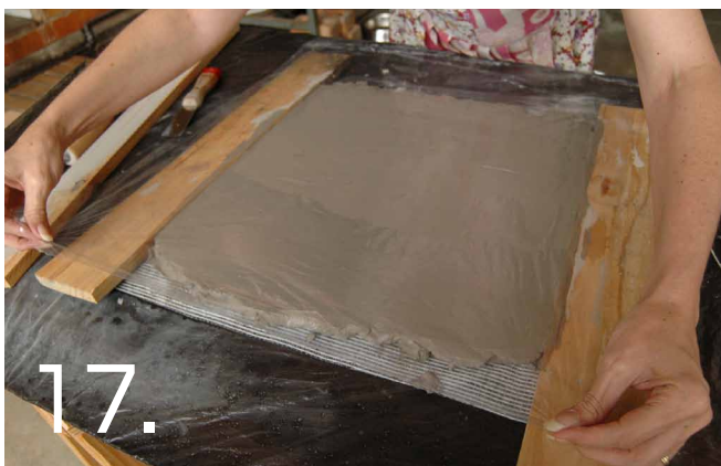
17. Lay a sheet of plastic over the surface. Smooth out air bubbles trapped under the plastic.
