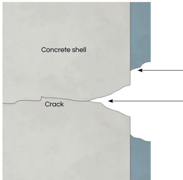
Remove PoolCrete (marble pool plaster) 75mm each side of crack through to concrete shell
